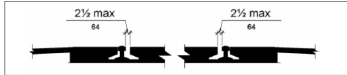
(Exception) Track Crossings
