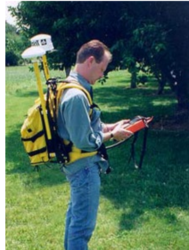
Backpack mounted GPS roving antenna and receiver unit
