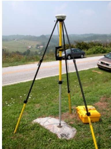
Survey grade GPS antenna mounted on tripod over a geodetic survey mark
