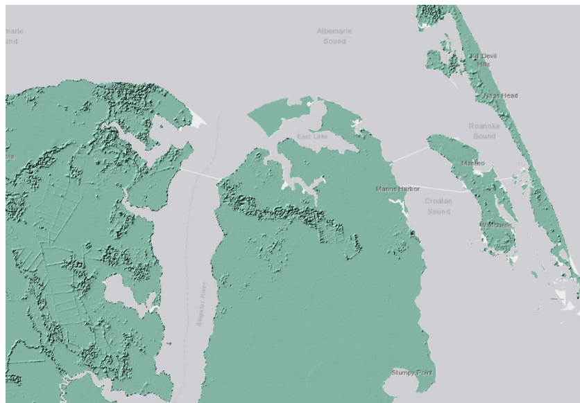
Digital Elevation Model of sound and coast off North Carolina (20 ft grid cell)
