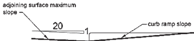
Counter Slope of Surfaces Adjacent to Curb Ramps
