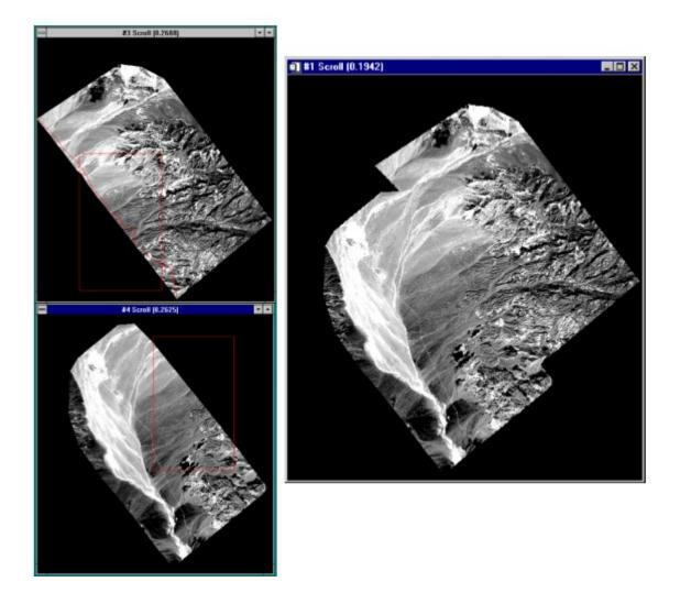
Above is an example of mosaicking in ENVI software. You can see the different scroll values on each of the image windows. These images can be linked to other images through geo-referencing. Most of the images we worked with were derived from satellites.
