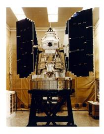
Landsat 4 was launched in 1982 and had significant changes from the previous three satellites. Landsat 4 had an improved sensor that could see better ground detail with a wider range. The Thematic Mapper took the place of the RBV instrument providing a larger spectral band. Landsat 4 was functional for nearly 20 years until it was finally decommissioned in 2001.
