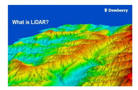
LiDAR differs from Radar primarily because it primarily uses optical signals which are near IR (infrared), while Radar uses microwave signals that have much longer wavelengths. The shorter wavelengths used by LiDAR allows for it to detect much smaller particles. One benefit of Radar is that it functions better than LiDAR with cloud coverage.
