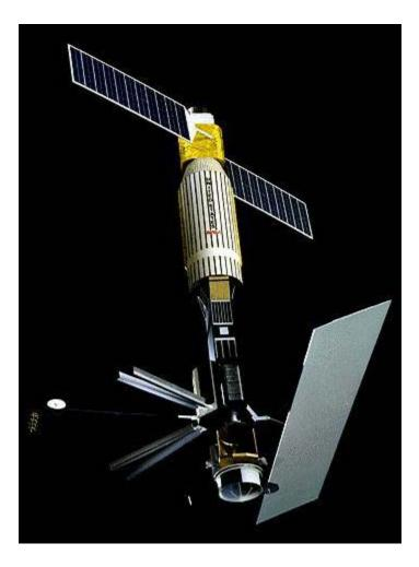
In October of 1978, the first AVHRR or Advanced Very High-Resolution Radiometer was launched. These space-borne sensors measure the earth's reflectance with five very wide spectral bands. Most of these sensors are carried and managed by NOAA. These sensors are primarily used to measure the earth's thermal emissions and cloud patterns.
