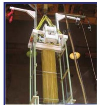
*Testing one of SuperPower's FCL modules*
