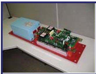
*Standard Building Block Assembly for the Silicon Power FCL*
