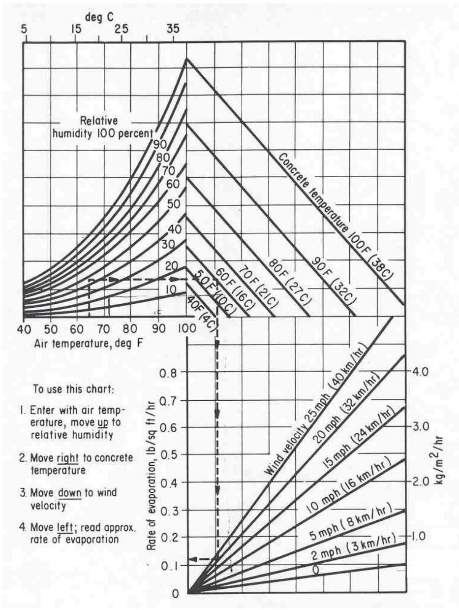
Figure 7. Chart. Evaporation rate nomograph from ACI 308.<sup>(4)</sup>
